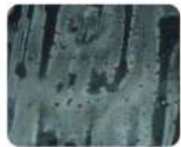
Deionized water control 0% soil removal Flash rust noted
