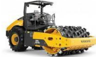
SHEEP'S FOOT COMPACTOR
